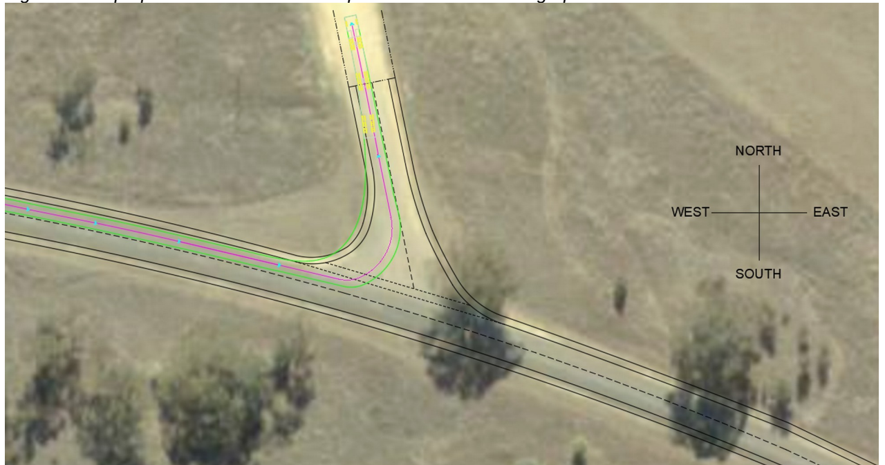
Figure 11: Superposition of B-Double Swept Path on Aerial Photograph
