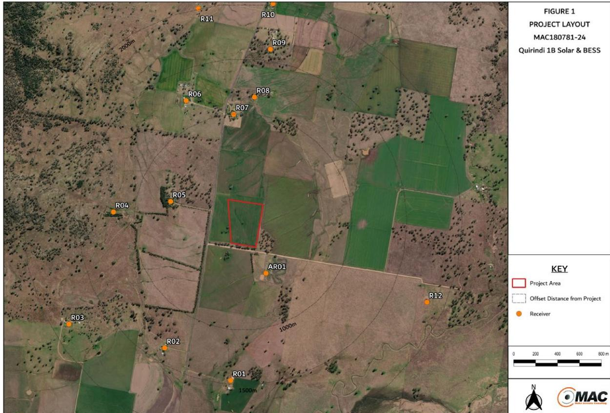
Figure 9: Location of noise sensitive receivers. Source: Muller Acoustic Consulting
